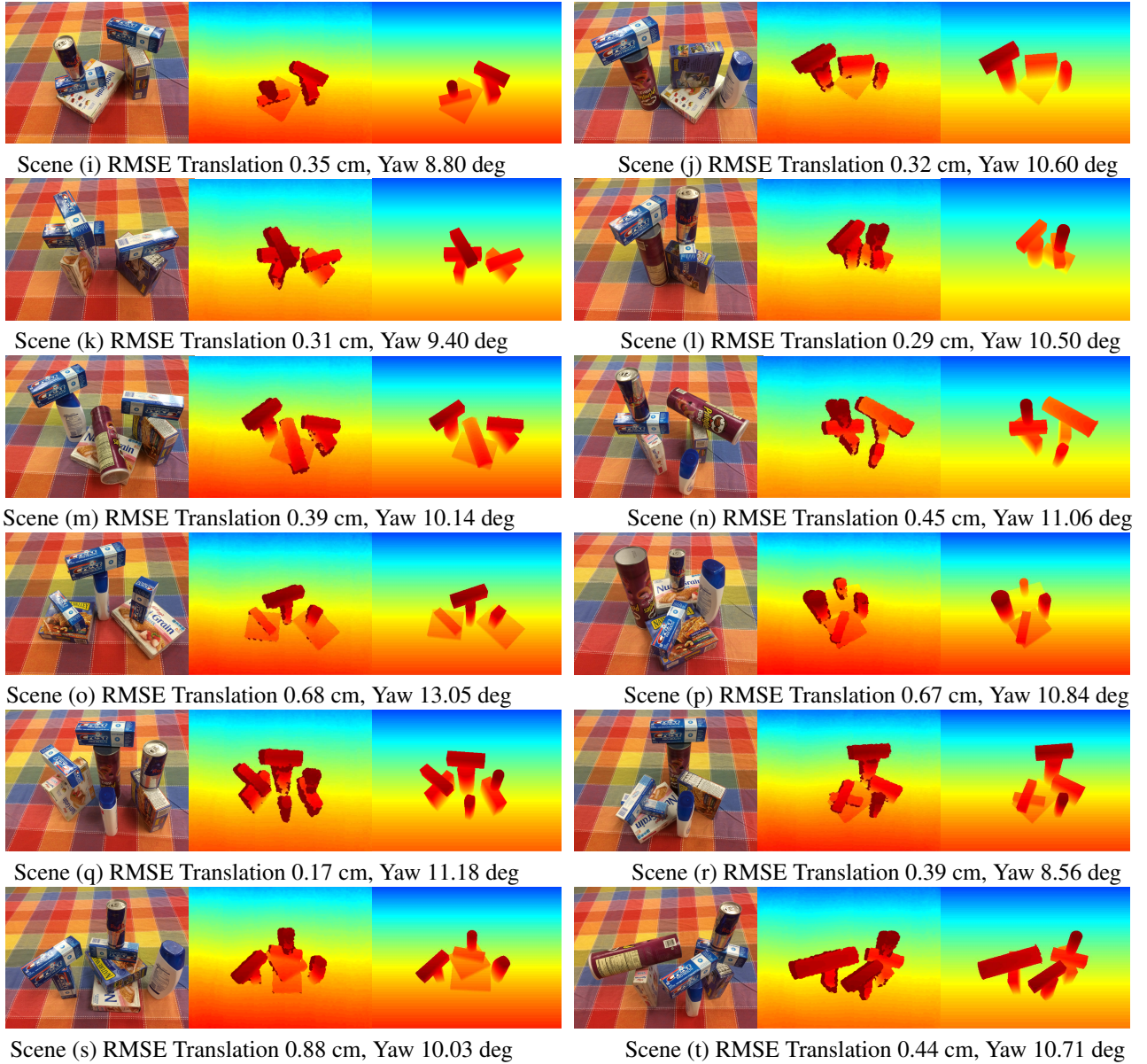
Figure 7. Pose estimation results for known axiom sets in scenes containing five to seven objects. Each subfigure, shows the RGB (left) and depth (middle) from an RGBD camera mounted on the head of the PR2 and estimated scene graph as a depth image (right), as well as the RMSE for translation and rotation error.
